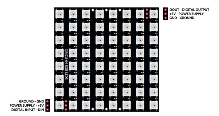
Note: Before connecting the pannel to any live (working) power supply, make sure that ground is always connected first before any other wire!
